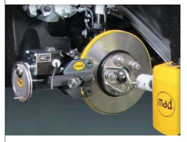
On Car Brake Lathe
